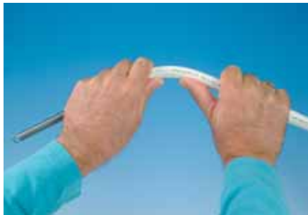
Bending with internal spiral spring
