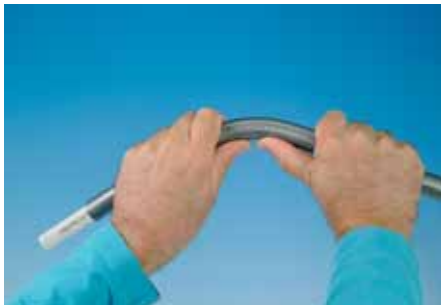
Bending with external spiral spring
